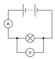
The ammeter reading is 2.0 A and the voltmeter reading is 6.0 V.
